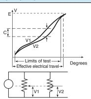
It is the maximum deviation between the actual voltage outputs of 2 or more pot modules in the same assembly. It is expressed as a percentage of the total applied voltage, or in dB attenuation.
